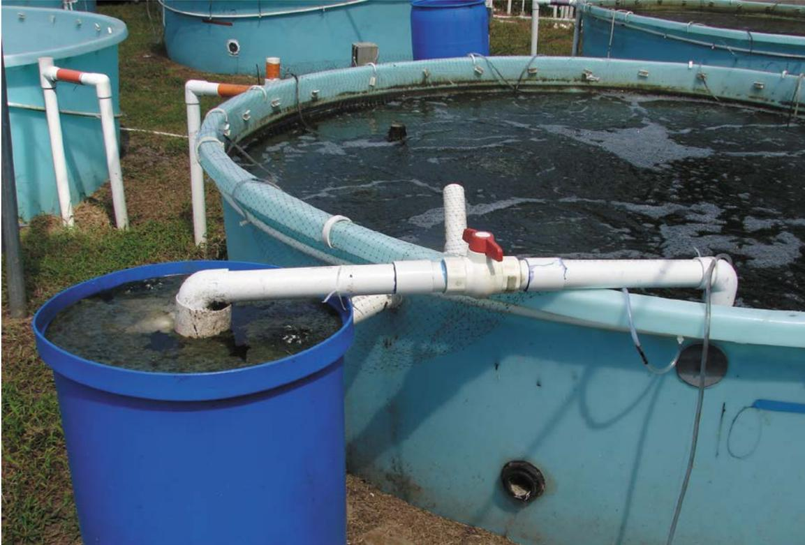
*\*A ceramic air diffuser located in the PVC pipe submerged in the shrimp culture tank moves water up the pipe and into the settling chamber. Water then enters a larger diameter pipe, causing velocity to slow. Particles settle on the bottom and clarified water at the surface of the settling chamber returns back to the shrimp culture tank.*
